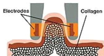
The special design headpiece uses vacuum to fold the skin, ensuring contact and positioning the dermis in direct alignment with radio frequency probe. The combination of this vacuum positioning and the use of RF concentrate heat deep in the dermis, leading to collagen contraction and regeneration.
